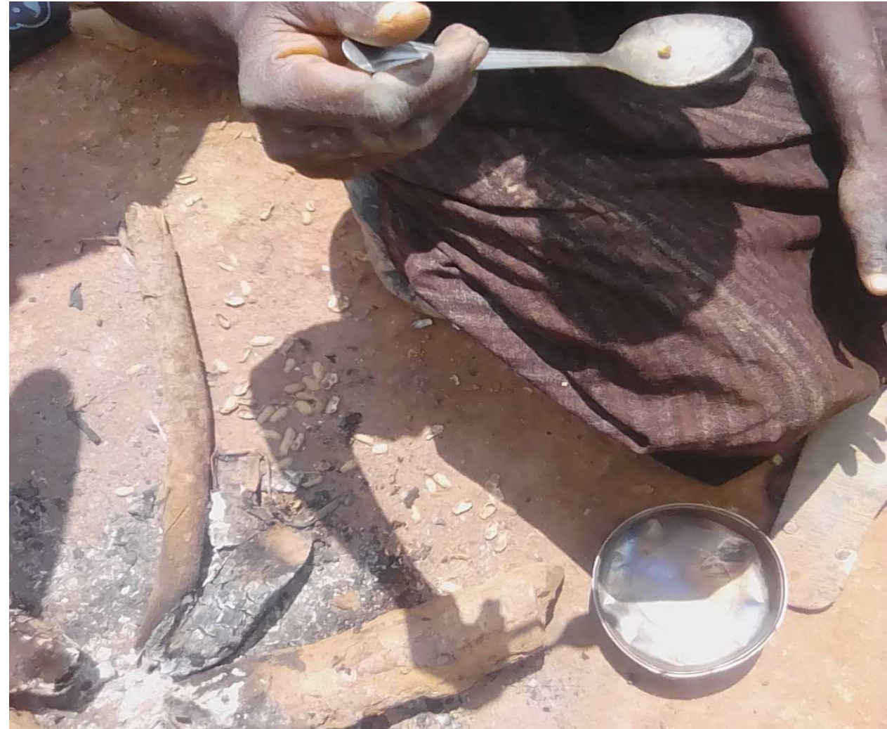
Open burning of Gold-mercury amalgam
