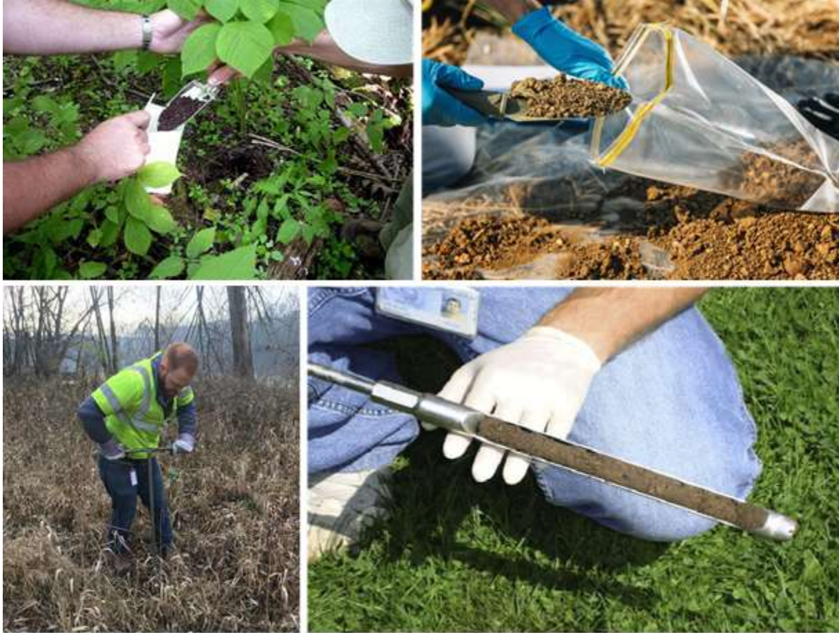
917 Figure 2: Commonly used soil samplers. Shovels (top), soil auger (bottom). Sources (in 918 clockwise order from the top left): Flickr, StockLib, Kim et al. (2012), Flickr.
