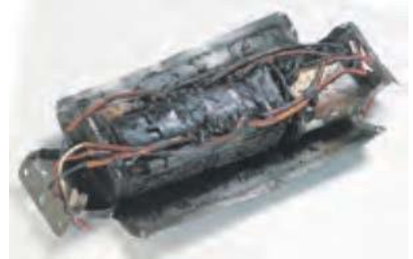
Fig. 10. Example of degraded ballast in a fluorescent light fixture
