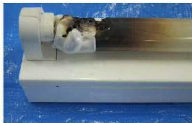
Fig. 9. Example of damage to a straight tube LED lamp
