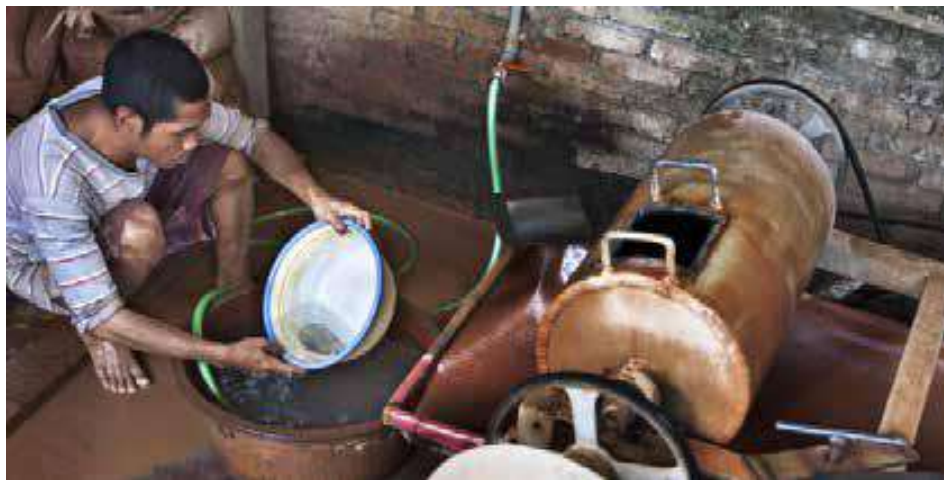
Figure-16: Excess Mercury Discharged to the Environment
