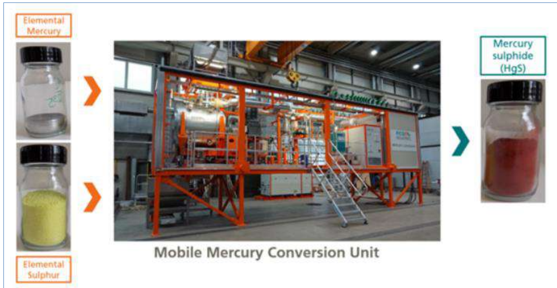
Figure-32: Stabilization Elemental Mercury into Mercury Sulfide
