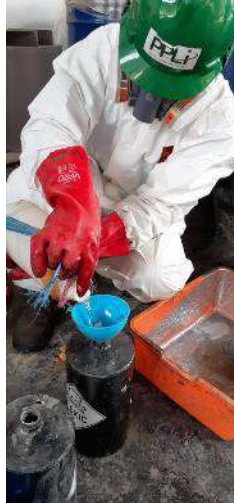
Figure-21: Re-packing of Liquid Elemental Mercury into Mercury Flask
