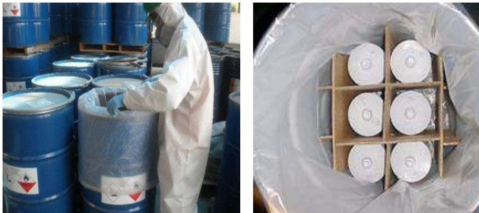
Figure-23: Over-packing of Evidence/Confiscated Elemental Mercury in Metal Drums
