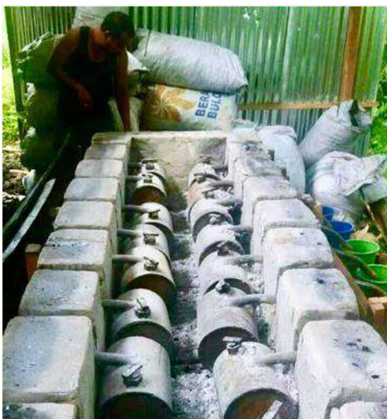
Figure-7: Mercury Distillation Process from Cinabar Ores
