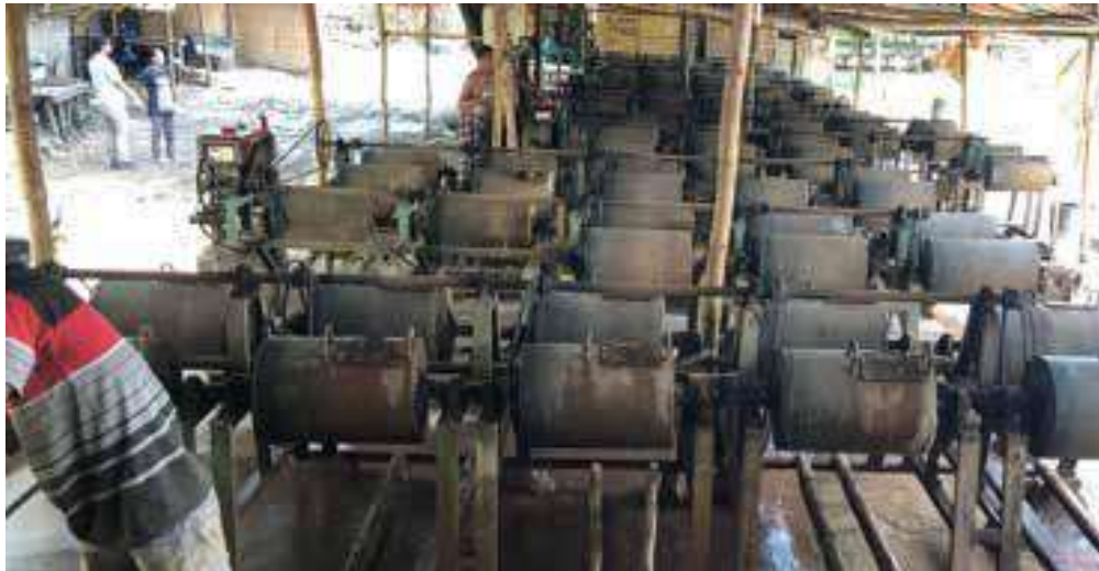
Figure-14: Gold Ore Grinding Process in Ballmills
