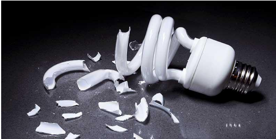
Figure 4-6: A broken CFL
