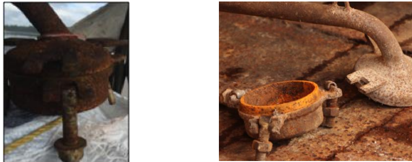
Figure 6-1 Type of retorts found at Potaro river dredges. Evidently with scarce use. (Photo Credit: Left: R. Romero, Right: C. Ohashi)
