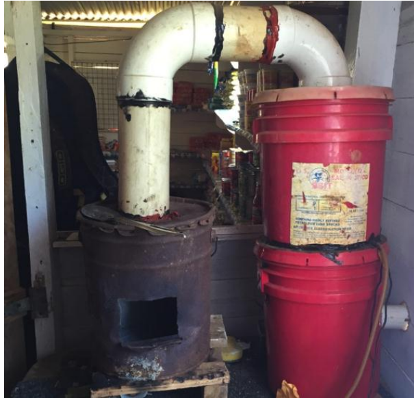
Figure VI-18. Retort adapted for indoor burning amalgam at Arakaka.
