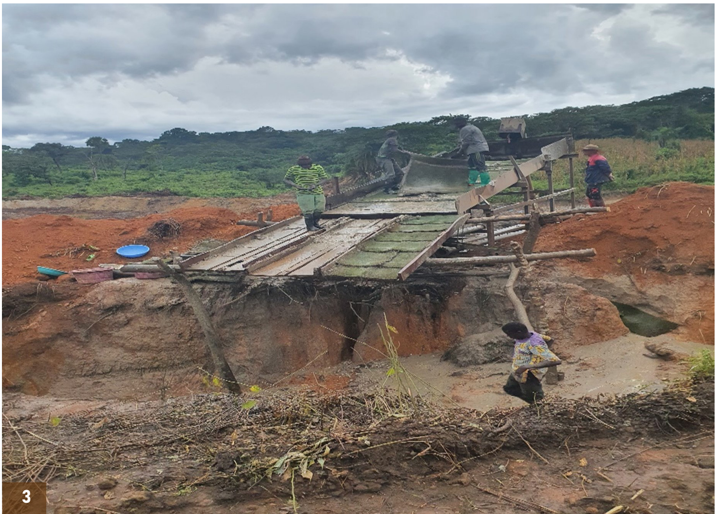
Figure 3: Treatment methods - (1) simple sluice in Djouzamie in Mbéré; (2) mechanical crushers in Kambélé in Kadey; (3) artisanal washing station in Bindiba in Lom and Djerem, (photos, MINMIDT 2022)
